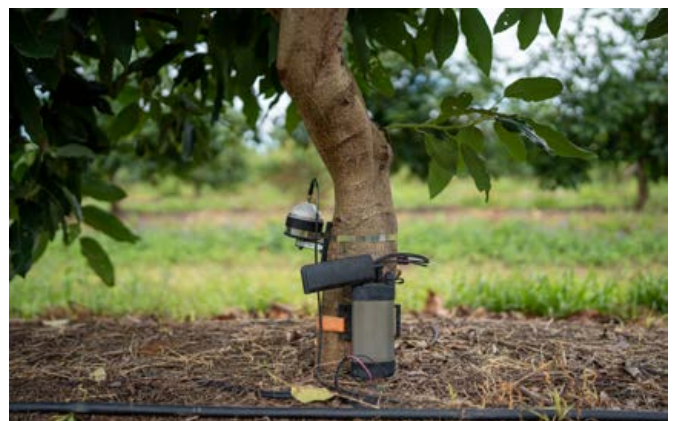
Dendrometers and sap flow meters at work in the Smart Farm.
